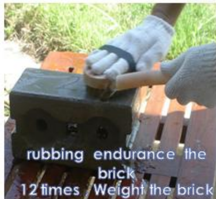
Give it to the 110 °C heating chamber for 2 days, Weight the brick
